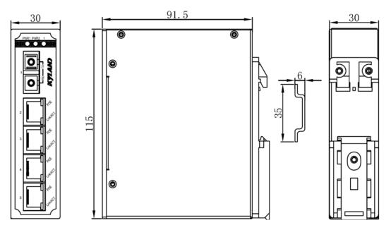
**♦** Dimension Drawing for Wall Mounting (Unit: mm)
