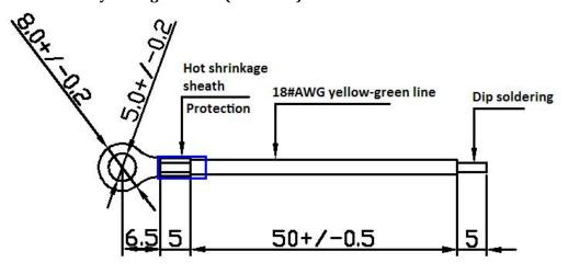
**Note**: If the KEIN1005S needs to do an insulated withstand voltage test, please disconnect the 18#AWG line to disable surge protection circuit, which will cause the failure of this experiment.
