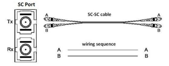
**Note**: A laser is used to transmit signals in fiber cables. The laser meets the requirements of level 1 laser products. Routine operation is not harmful to your eyes, but do not look directly at the fiber port and fiber connector when the switch is powered on.
