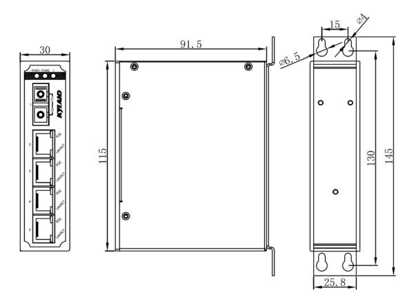
**Note**: The switch housing is a part of the heat dissipation system, which becomes hot during operation. Please be careful when handling the device during operation.
