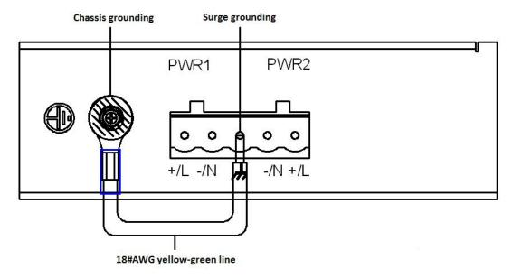
There is a grounding screw on the top panel of the KIEN1005S, which is for chassis
