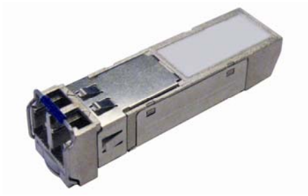
Figure 15: 1000Base SFP fiber module
