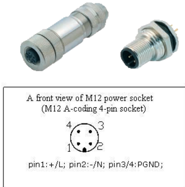
Figure 3-6 Wiring sequence of M12 power input terminal
